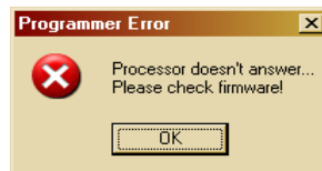
Illustration 3: Firmware is missing in the programmer
